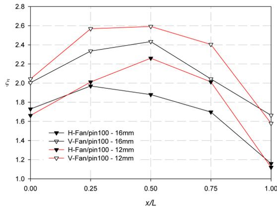
Fig. 7. Heat transfer enhancement by vertical and horizontal piezofans of the present 10-mm-high pin-fin heat sink with fan heights of 12 mm and 16 mm.
