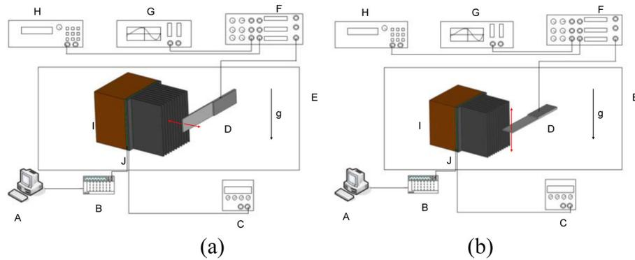
Fig. 1. The present experimental setup having (a) a vertical piezofan, and (b) a horizontal piezofan on a tested heat sink; the red arrow indicates the piezofan vibration direction, and the black arrow indicates gravity.
