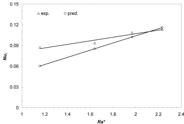
Fig. 4. Comparison of natural convection heat transfer of 10-mm-high plate-fin heat sink between the present measurement and the calculated value by the correlation proposed by Van De Pol and Tierney.
