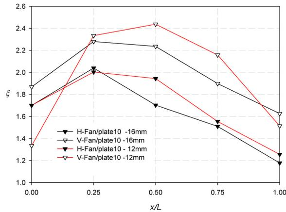
Fig. 6. Heat transfer enhancement by vertical and horizontal piezofans of the present 10-mm-high plate-fin heat sink with fan heights of 12 mm and 16 mm.
