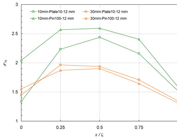
Fig. 5. Heat transfer enhancement of 10-mm-high and 30-mm-high heat sinks with a vertical piezofan at various fan positions.
