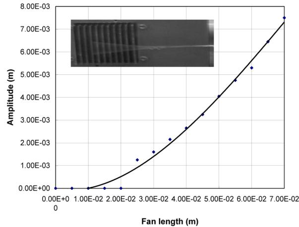
Fig. 3. Displacement of the present 70-mm-long vibrating piezofan at different positions operated at resonant frequency.
