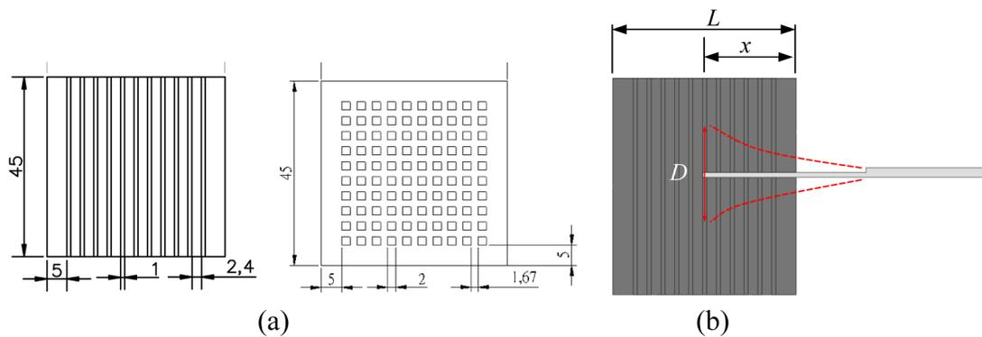
Fig. 2. Schematic diagrams of (a) present plate-fin heat sink having 11 plates and pin-fin heat sink having 100 square pins, (b) a piezofan having horizontal vibration over a heat sink and the definition of both  $x$  and  $L$ .
