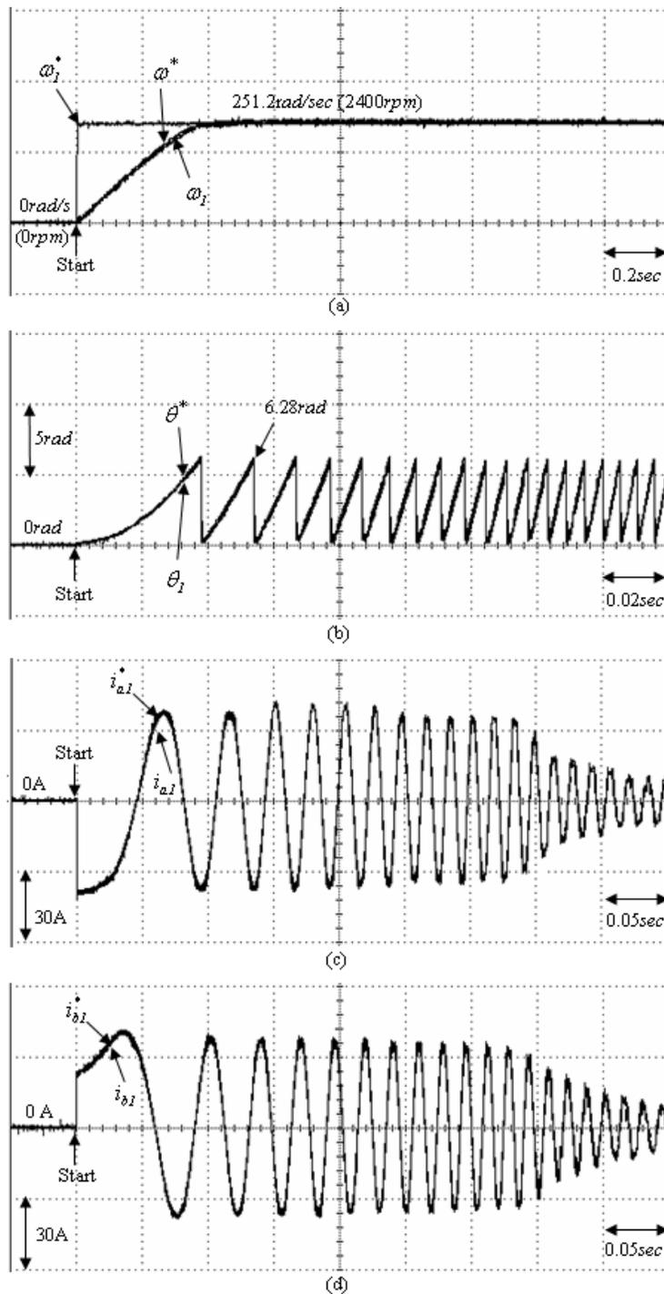
Fig. 7. Experimental results of the proposed novel hybrid modified Elman NN controlled for a PMSM drive electric scooter at 251.2 rad/sec (2400 rpm): (a) command rotor speed  $\omega_1^*$ , desired rotor speed  $\omega^*$  and measured rotor speed  $\omega_1$ ; (b) command rotor position  $\theta^*$ , measured rotor position  $\theta_1$ ; (c) command current  $i_{a1}^*$  and measured current  $i_{a1}$  in phase a1; (d) command current  $i_{b1}^*$  and measured current  $i_{b1}$  in phase b1.
