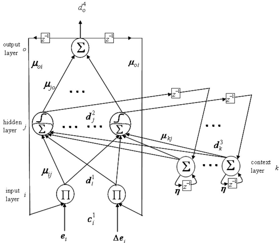
Fig. 3. Structure of the four-layer modified Elman NN.
