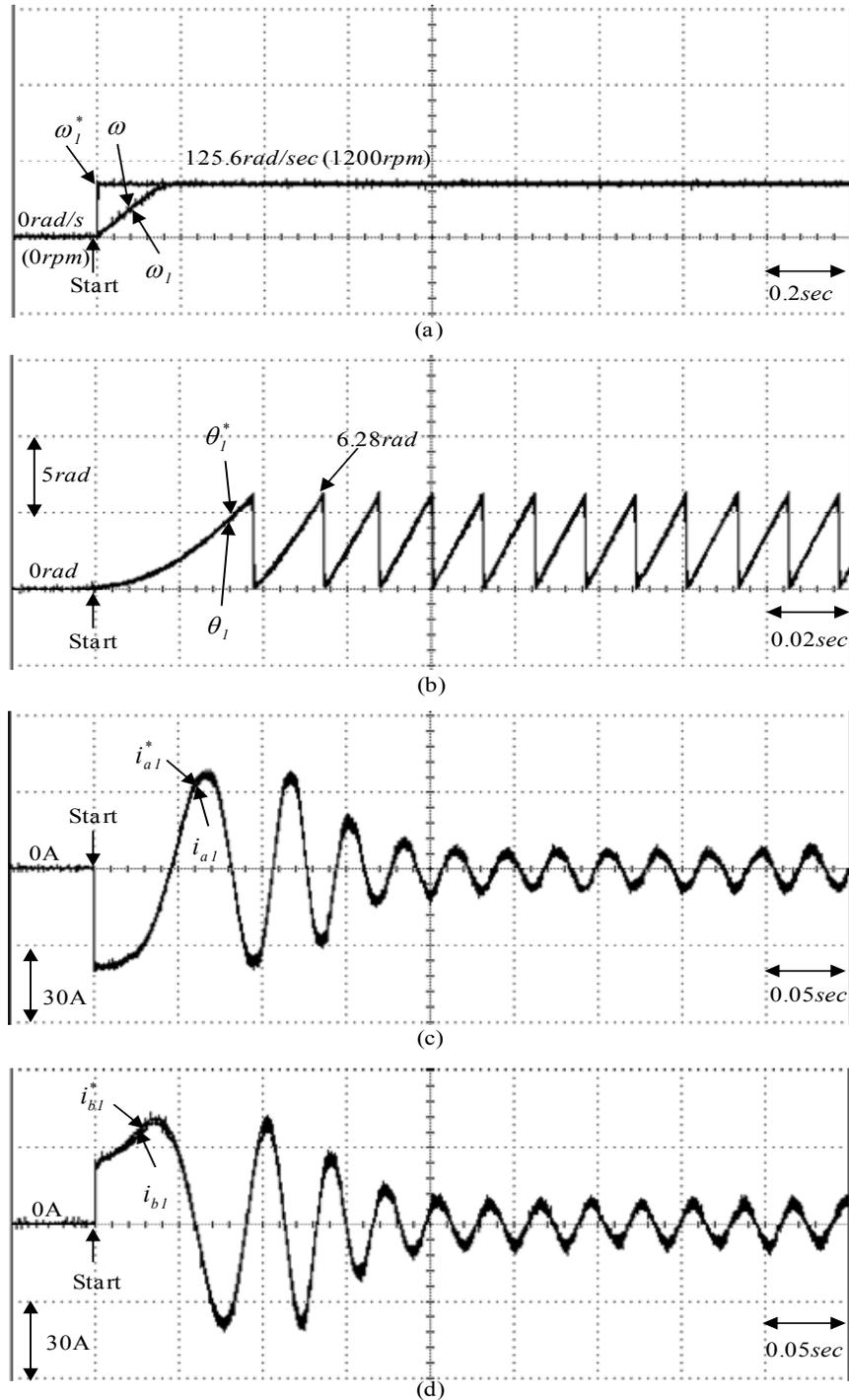
Fig. 6. Experimental results of the proposed novel hybrid modified Elman NN controlled for a PMSM drive electric scooter at 125.6 rad/sec (1200 rpm): (a) command rotor speed  $\omega_1^*$ , desired rotor speed  $\omega^*$  and measured rotor speed  $\omega_1$ ; (b) command rotor position  $\theta_1^*$ , measured rotor position  $\theta_1$ ; (c) command current  $i_{a1}^*$  and measured current  $i_{a1}$  in phase a1; (d) command current  $i_{b1}^*$  and measured current  $i_{b1}$  in phase b1.
