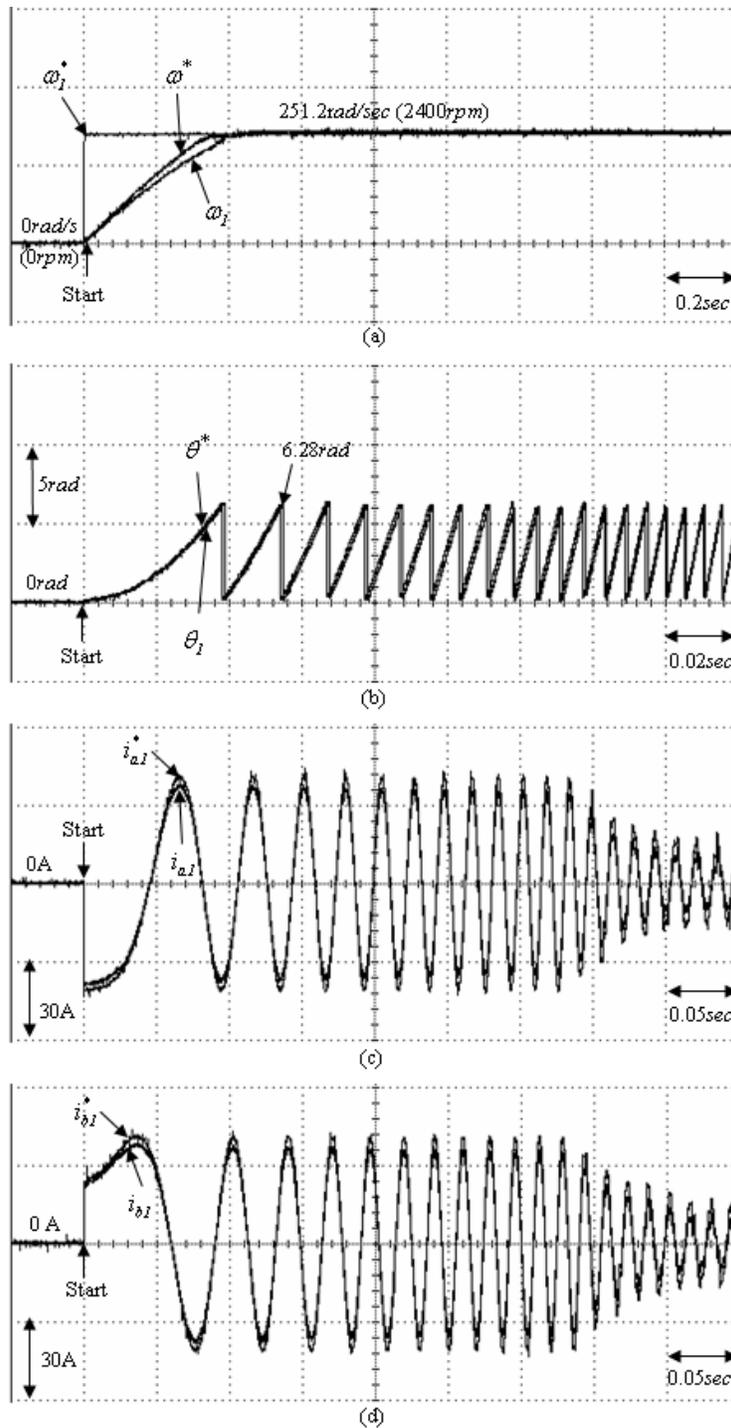
Fig. 5. Experimental results of the PI controlled for a PMSM drive electric scooter at 251.2 rad/sec (2400 rpm): (a) command rotor speed  $\omega_1^*$ , desired rotor speed  $\omega^*$  and measured rotor speed  $\omega_1$ ; (b) command rotor position  $\theta^*$ , measured rotor position  $\theta_1$ ; (c) command current  $i_{a1}^*$  and measured current  $i_{a1}$  in phase a1; (d) command current  $i_{b1}^*$  and measured current  $i_{b1}$  in phase b1.
