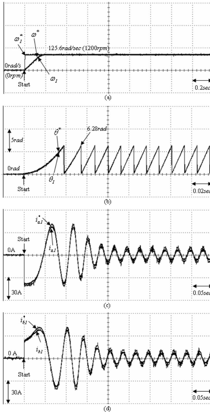
Fig. 4. Experimental results of the PI controlled for a PMSM drive electric scooter at 125.6 rad/sec (1200 rpm): (a) command rotor speed  $\omega_1^*$ , desired rotor speed  $\omega^*$  and measured rotor speed  $\omega_1$ ; (b) command rotor position  $\theta^*$ , measured rotor position  $\theta_1$ ; (c) command current  $i_{a1}^*$  and measured current  $i_{a1}$  in phase a1; (d) command current  $i_{b1}^*$  and measured current  $i_{b1}$  in phase b1.
