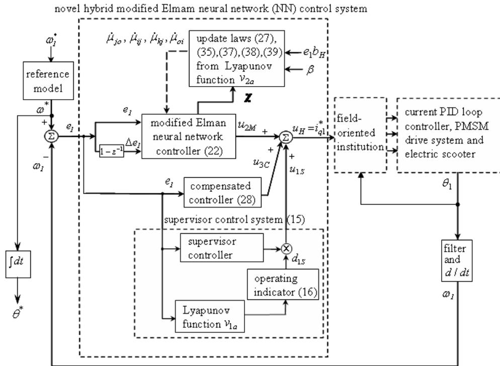
Fig. 2. Block diagram of novel hybrid modified Elman NN control system.
