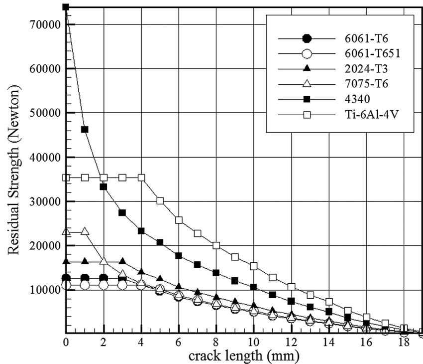
Fig. 10. The relationship between the overall residual strength and the crack length of various materials, considering the influence of static strength.
