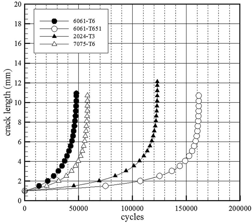
Fig. 7. The relationship between the crack length and the life cycles of various aluminum alloys, under load.
