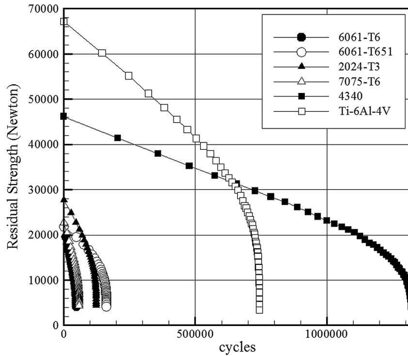
Fig. 9. The relationship between the residual strength and the load cycle number of various materials.
