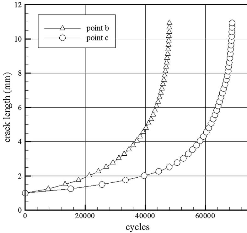
Fig. 5. The relationship between crack length and the life cycles at various positions, under load.
