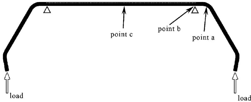
Fig. 2. The loads and specified positions of the initial cracks (points a, b and c).
