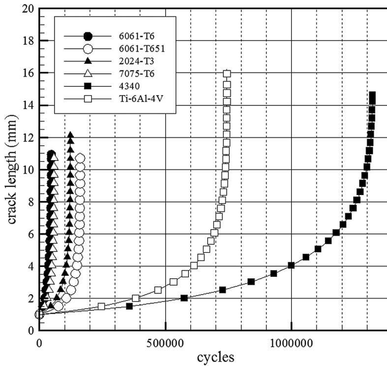
Fig. 6. The relationship between the crack length and the life cycles of different materials, under load.
