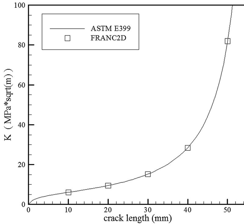
Fig. 3. A comparison of the results provided by FRANC2D and the ASTM standard.
