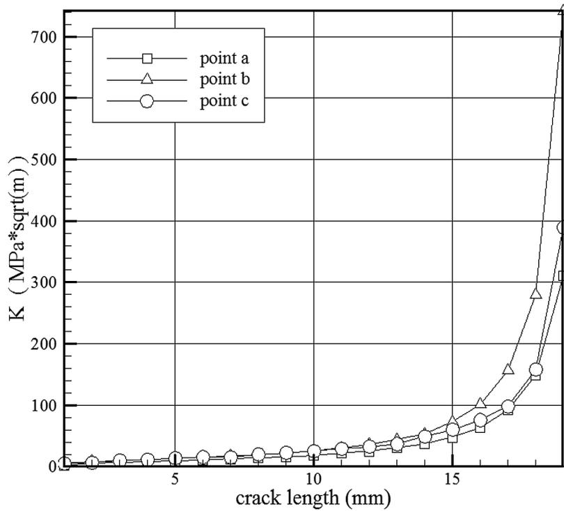
Fig. 4. The relationship between the SIF and the crack length at various positions, under load.
