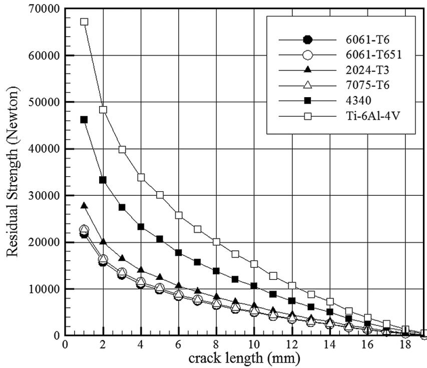
Fig. 8. The relationship between the residual strength and the crack length of various materials.
