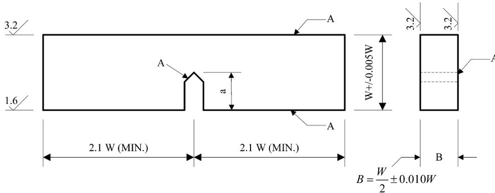
Fig. 1. SENB based on ASTM E399-09 [17].
