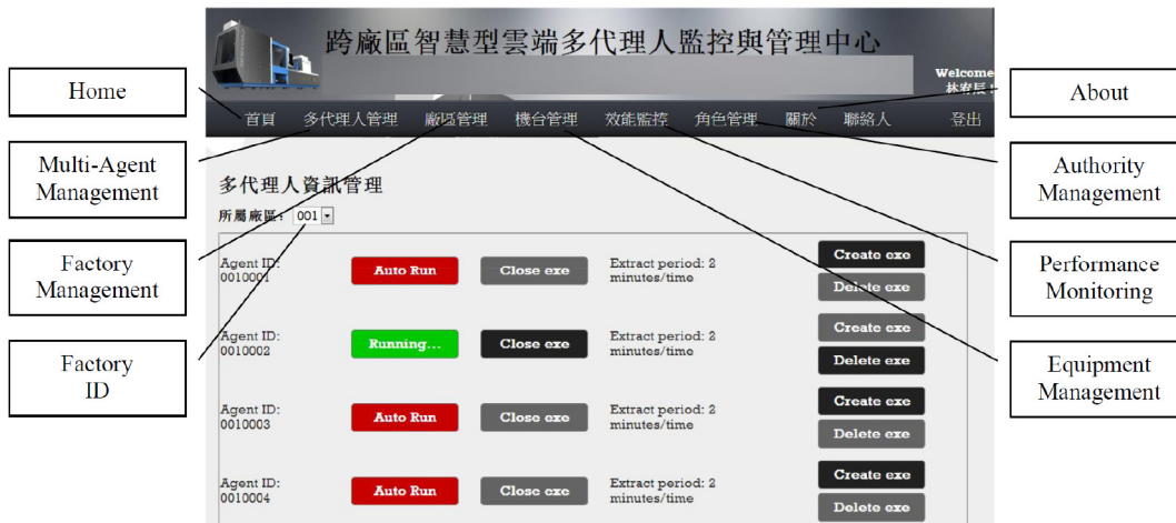
Fig. 2. Injection molding machine manufacturing monitoring system interface.
