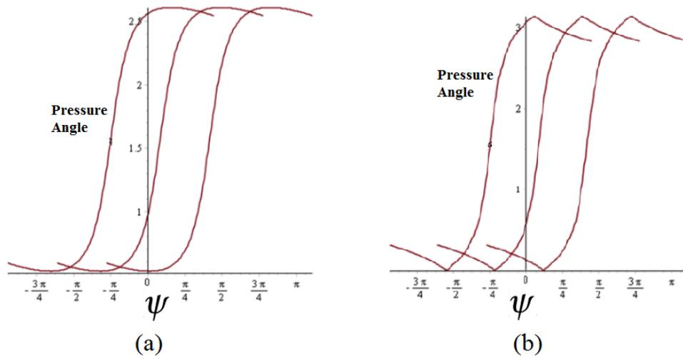
Fig. 6. Pressure angle for negative action with: (a)  $M = 3$ ,  $N = 4$ ,  $\alpha_3 = \tan^{-1}(M/N) - 0.0174$ ; (b)  $M = 3$ ,  $N = 4$ ,  $\alpha_3 = \tan^{-1}(M/N) - 0.0348$ .
