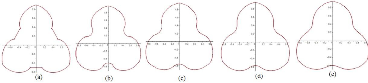
Fig. 1. Cam-profiles for three lobes: (a) one roller, (b) two rollers, (c) three rollers, (d) four rollers, (e) five rollers.
