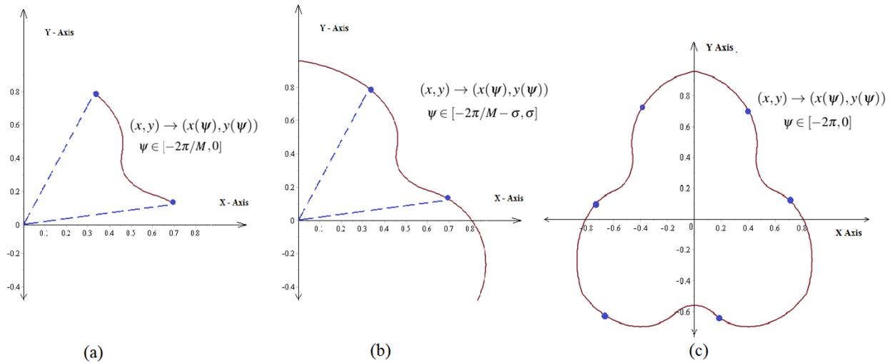
Fig. 3. (a) Complete pitch curve of the cam-profile when projected onto the X-Y plane; (b) complete cam-profile in two dimensions; (c) conical surface defining the spherical cam-profile intersecting the sphere on which the spherical mechanism is based.
