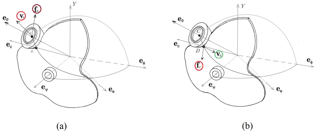
Fig. 5. Illustration of the pressure angle: (a) positive action; (b) negative action.
