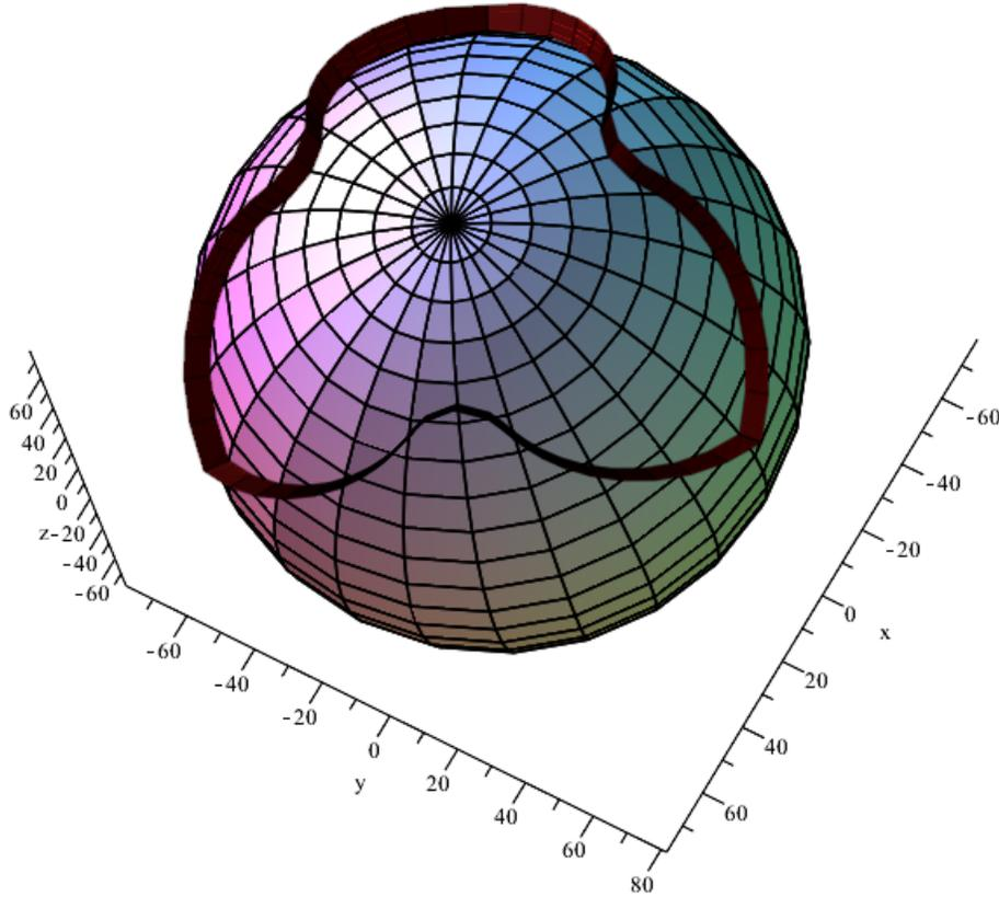
Fig. 4. The three dimensional plot of the conical surface that defines the spherical cam-profile intersecting the sphere on which the spherical mechanism is based.
