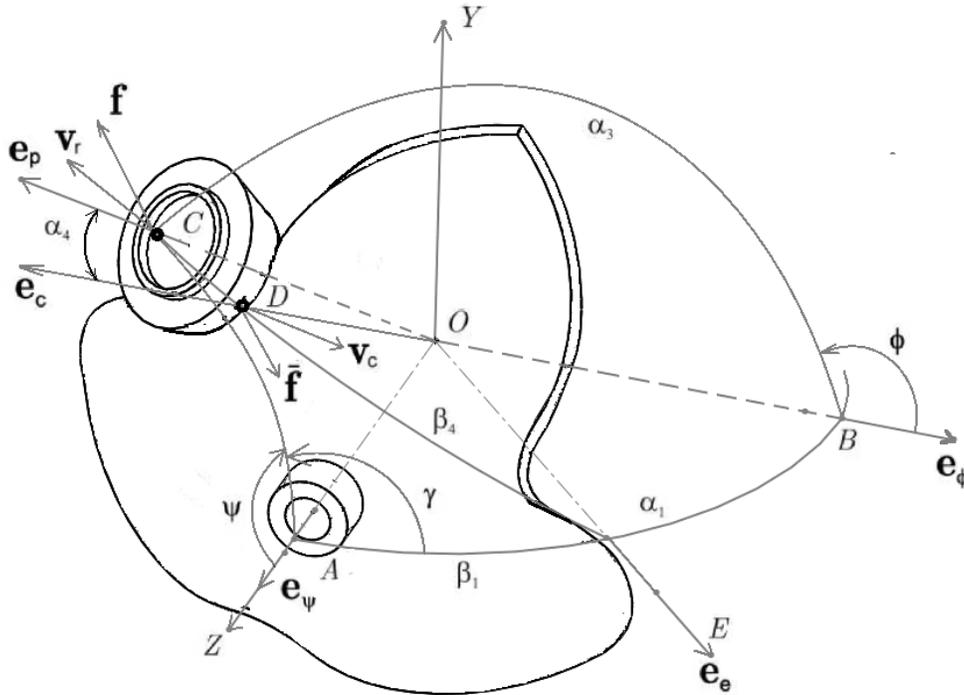
Fig. 2. Axes and angles defined for the spherical cam mechanism.
