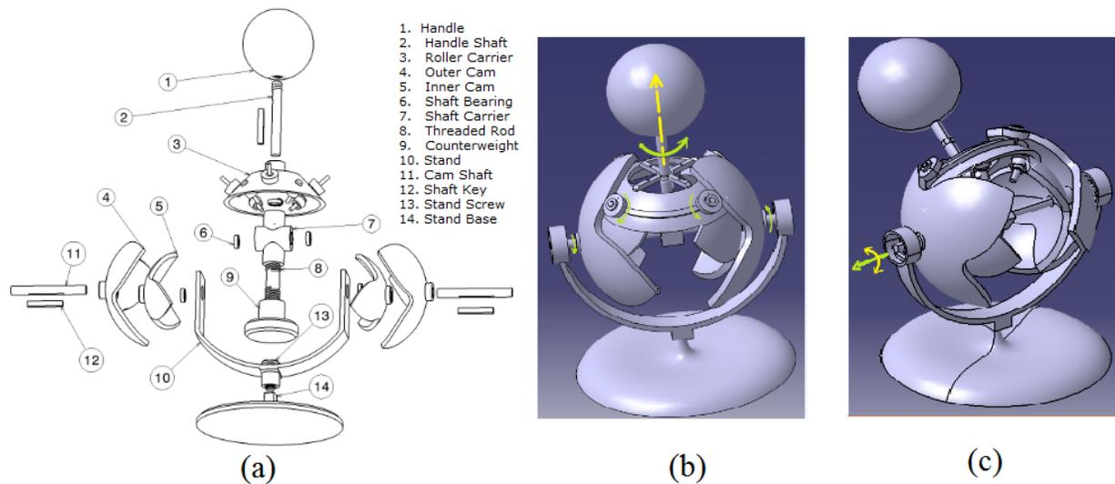
Fig. 7. (a) Exploded view of the joystick assembly; (b) Illustration of the roll motion; (c) Illustration of pitching motion of the joystick.
