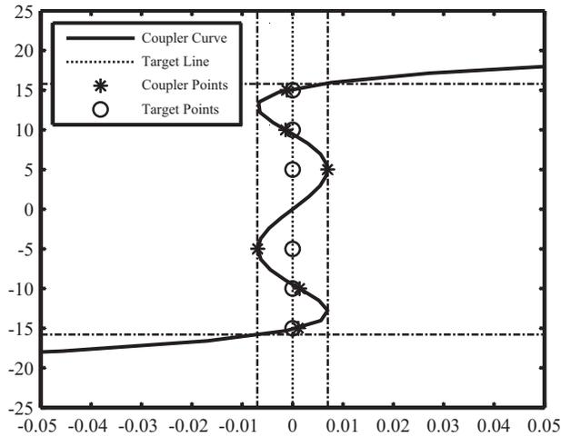
Fig. 6. Optimized coupler curve with six target points.
