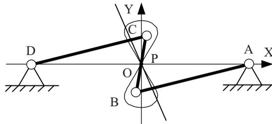
Fig. 4. Diagram of modified Watt's linkage.
