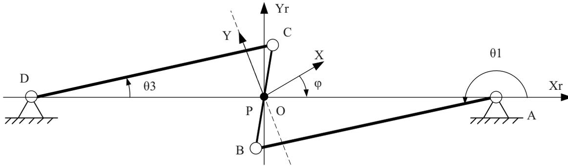
Fig. 5. Modified Watt's linkage with its design variables.
