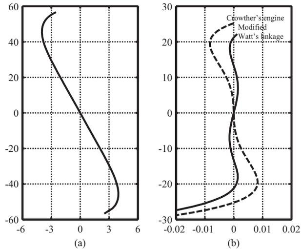
Fig. 3. The path of  $P$  in modified Watt's linkage.
