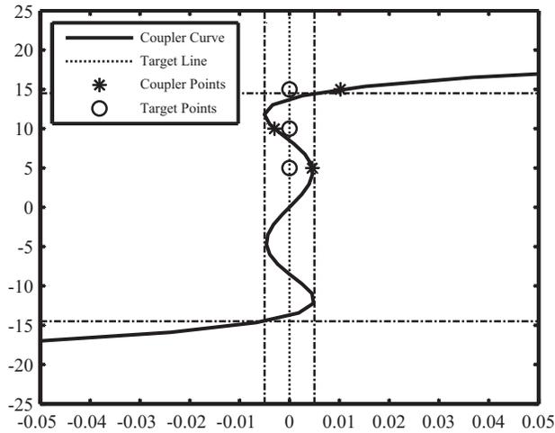
Fig. 7. Optimized coupler curve with three target points.
