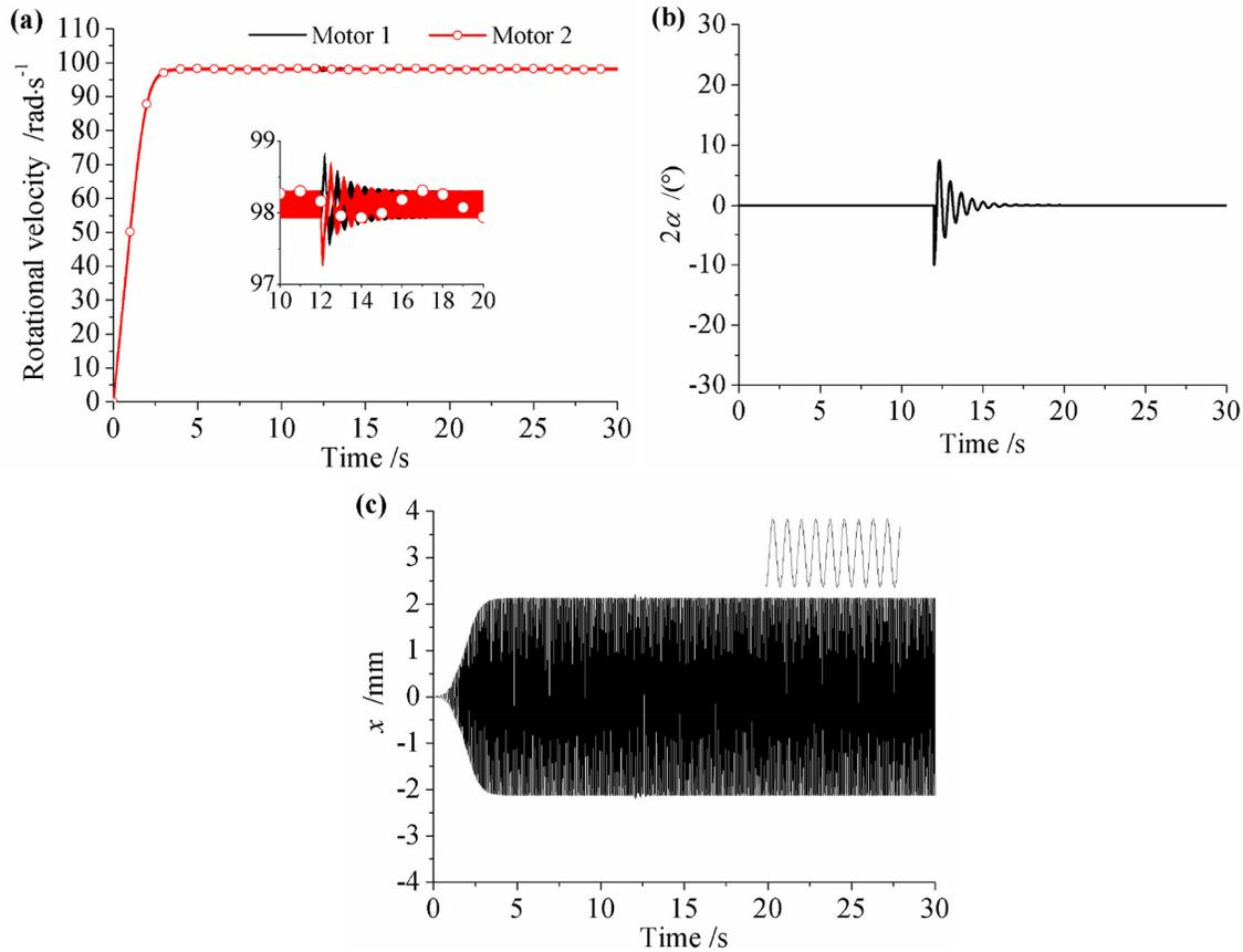
Fig. 4. Simulation results of two identical REMs in a sub-resonant state ( $k_x = 2.0 \times 10^7$ ,  $\Delta k_x = 1.5 \times 10^7$ ). (a) Rotational velocities of two REMs; (b) phase difference between two REMs ( $2\alpha = \varphi_1 - \varphi_2$ ); (c) displacement in  $x$ -direction.
