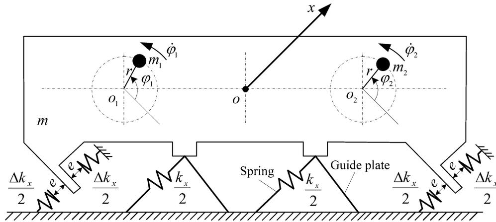
Fig. 1. Dynamical model of a nonlinear vibrating system.
