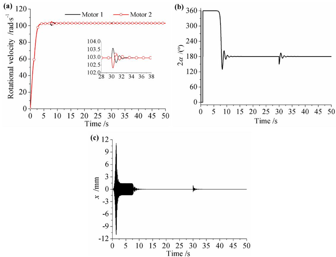
Fig. 5. Simulation results of two identical REMs in a super-resonant state ( $k_x = 6.26 \times 10^6$ ,  $\Delta k_x = 2.0 \times 10^6$ ). (a) Rotational velocities of two REMs; (b) phase difference between two REMs ( $2\alpha = \varphi_1 - \varphi_2$ ); (c) displacement in  $x$ -direction.
