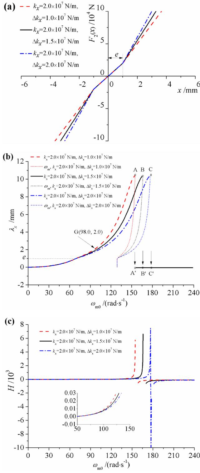
Fig. 2. Dynamical characteristic of the vibrating system versus  $\Delta k_x$  under the condition of  $k_x = 2.0 \times 10^7$  N/m. (a) Restoring forces of springs versus displacements; (b) frequency-amplitude relationship in the steady state; (c) coefficient of ability of stability.
