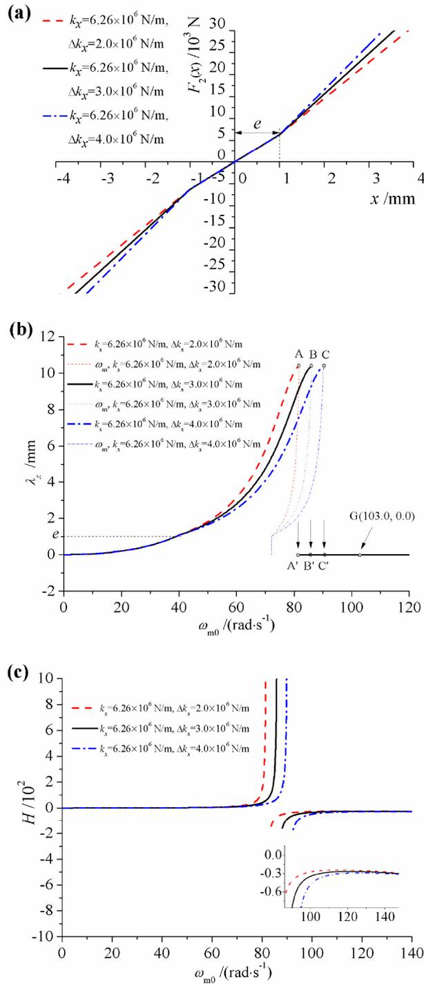
Fig. 3. Dynamical characteristic of the vibrating system versus  $\Delta k_x$  under the condition of  $k_x = 6.26 \times 10^6$  N/m. (a) Restoring forces of springs versus displacements; (b) frequency-amplitude relationship in the steady state; (c) coefficient of ability of stability.
