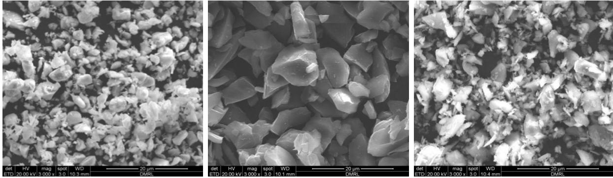
Fig. 1. (a) SEM picture of  $ZrB_2$  powder; (b) SEM picture of  $B_4C$  powder; (c) SEM picture of  $SiC$  powder.
