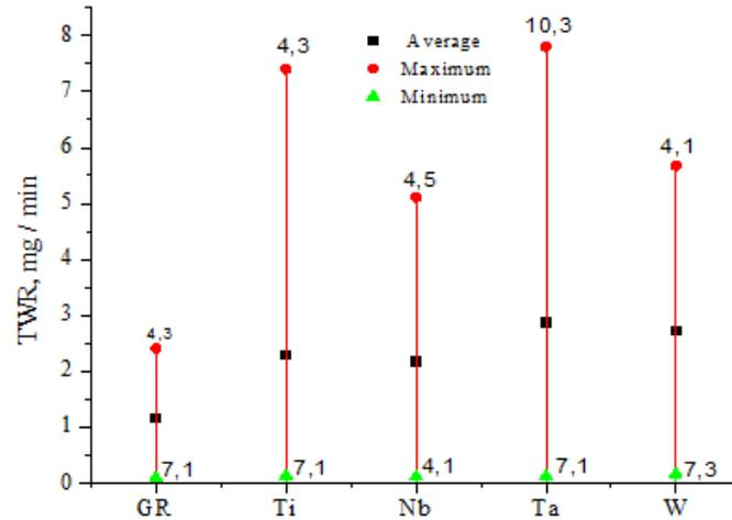
Fig. 14. TWR vs. tool at different pulse conditions for 70% ZrB<sub>2</sub>-30% SiC.
