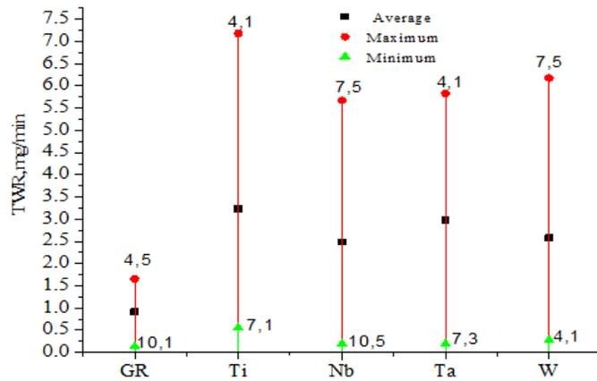
Fig. 12. TWR vs. tool at different pulse conditions for 80% ZrB<sub>2</sub>-20% SiC.
