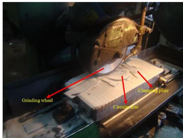
Fig. 3. Grinding of the workpiece.
