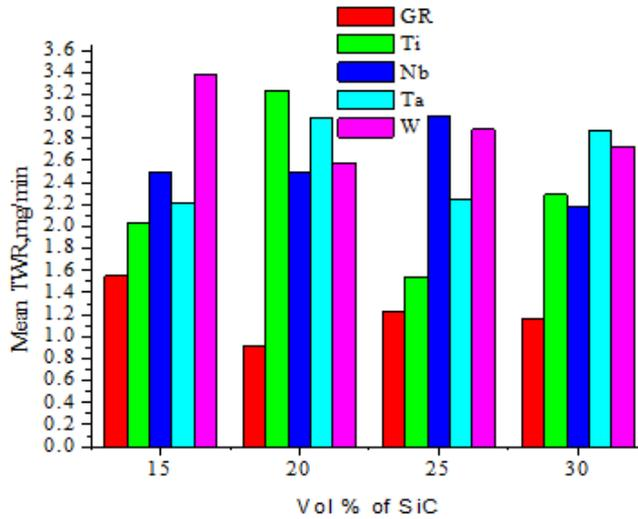
Fig. 15. Mean TWR Imparted by work material.
