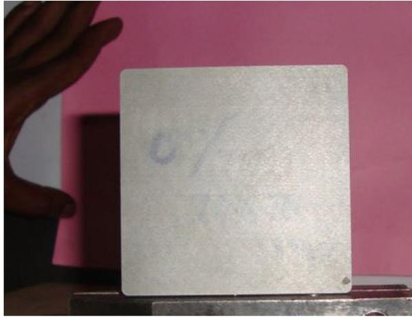
Fig. 4. Workpiece after grinding and square cut.
