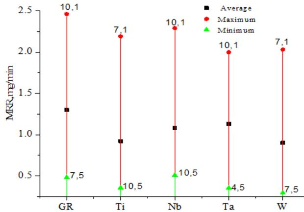
Fig. 20. MRR vs. tool at different pulse conditions for 75% ZrB<sub>2</sub>-25% SiC.
