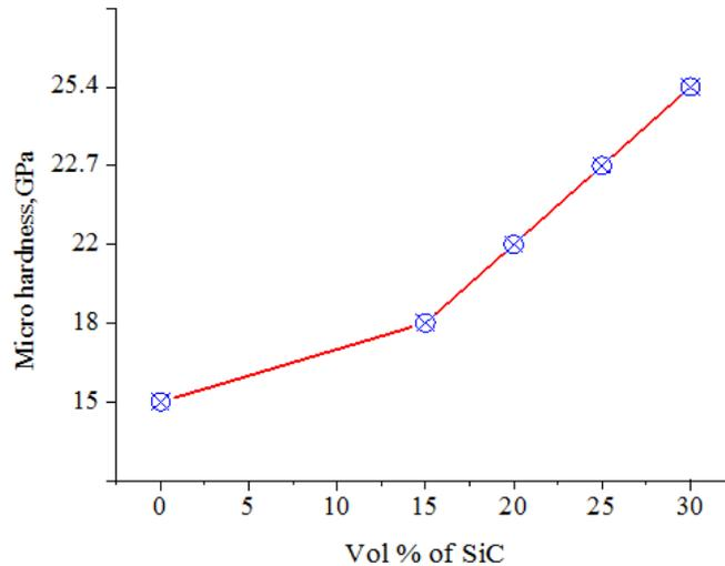
Fig. 8. Micro hardness with different Vol. % SiC.
