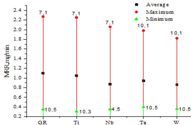
Fig. 18. MRR vs. tool at different pulse conditions for 85% ZrB<sub>2</sub>-15% SiC.
