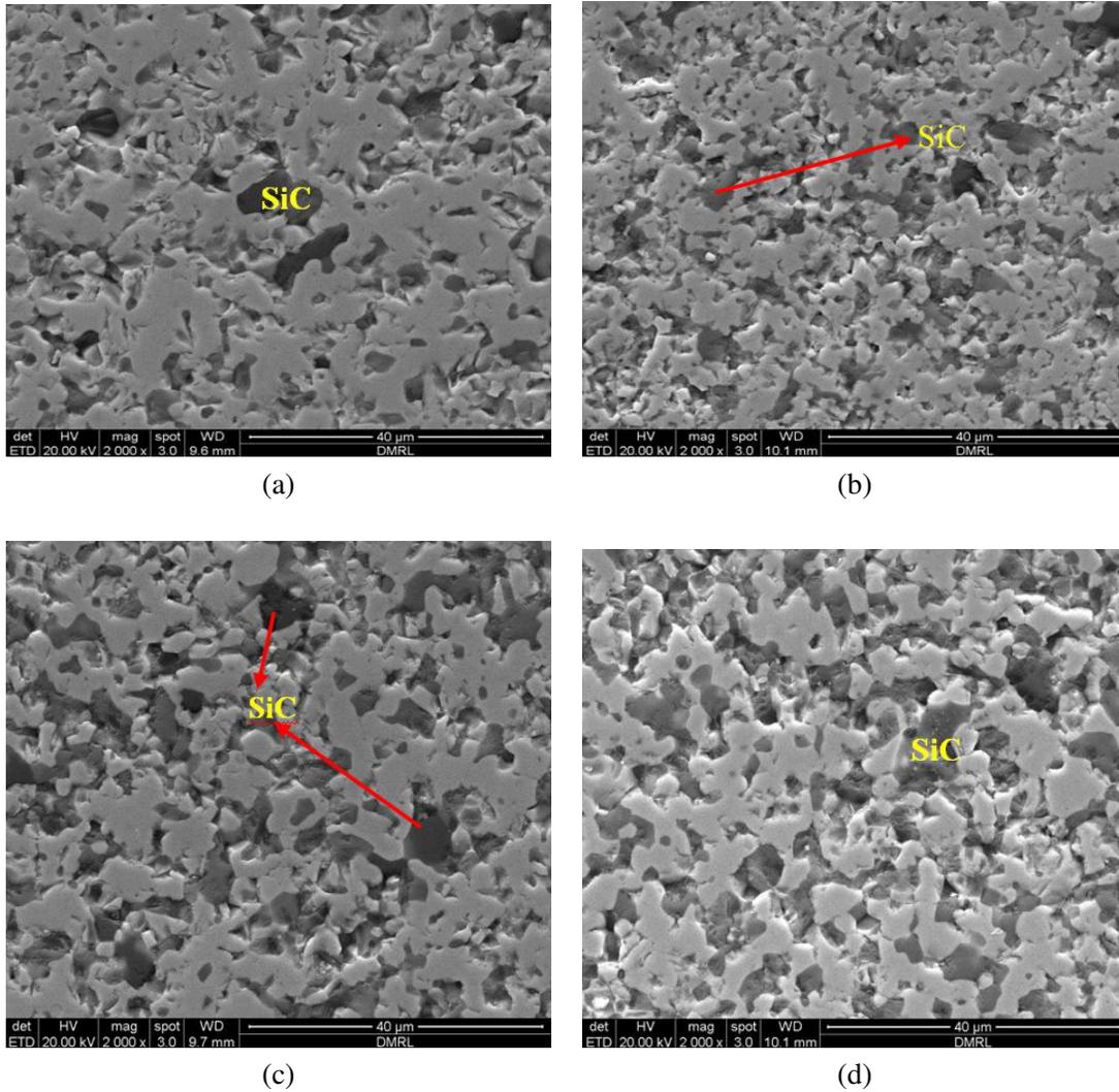
Fig. 7. (a) SEM picture of 85% ZrB<sub>2</sub>-15% SiC; (b) SEM picture of 80% ZrB<sub>2</sub>-20% SiC; (c) SEM picture of 75% ZrB<sub>2</sub>-25% SiC; (d) SEM picture of 70% ZrB<sub>2</sub>-30% SiC.
