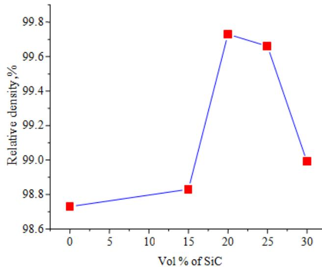
Fig. 5. Relative density of composite with different Vol.% of SiC.
