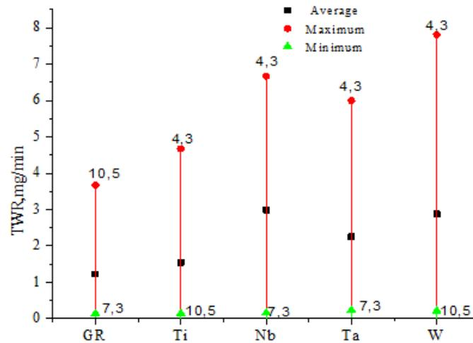
Fig. 13. TWR vs. tool at different pulse conditions for 75% ZrB<sub>2</sub>-25% SiC.
