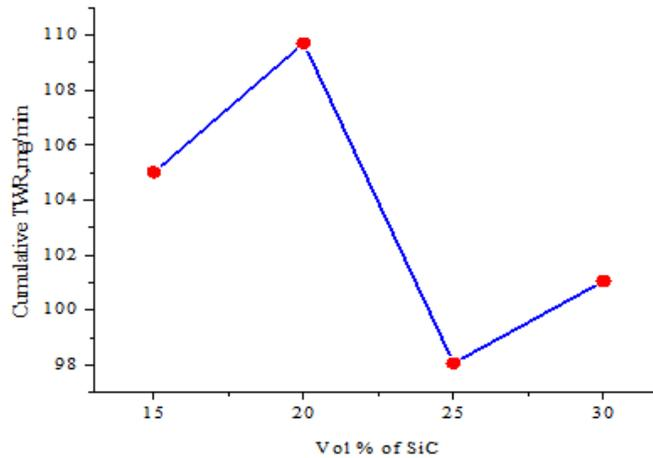
Fig. 16. Cumulative TWR for different Vol. % of SiC.
