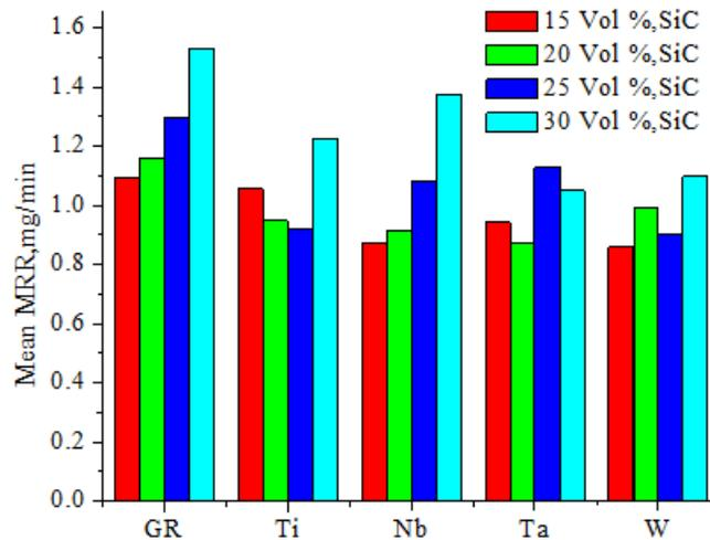
Fig. 22. Mean MRR imparted by tool material.
