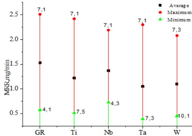
Fig. 21. MRR vs. tool at different pulse conditions for 70% ZrB<sub>2</sub>-30% SiC.
