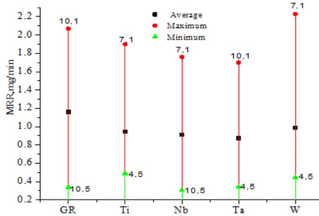
Fig. 19. MRR vs. tool at different pulse conditions for 80% ZrB<sub>2</sub>-20% SiC.
