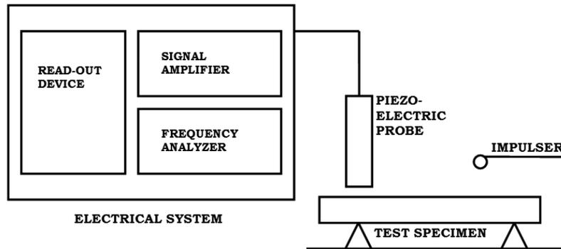
Fig. 9. Schematic of the dynamic modulus measurement system.
