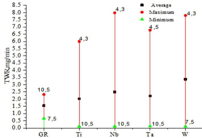
Fig. 11. TWR vs. tool at different pulse conditions for 85% ZrB<sub>2</sub>-15% SiC.
