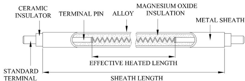
Fig. 1. Structure of the electric heater.
