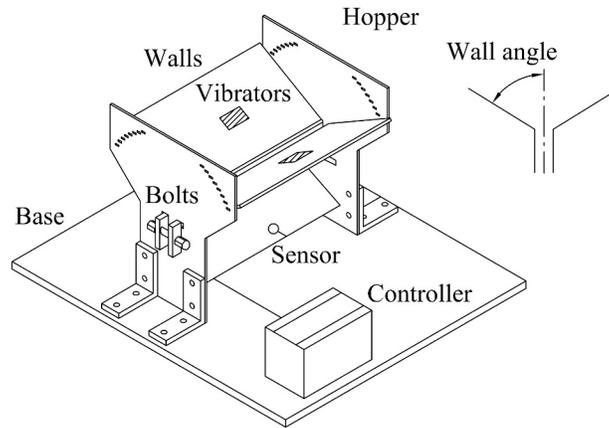
Fig. 2. Experimental apparatus.
