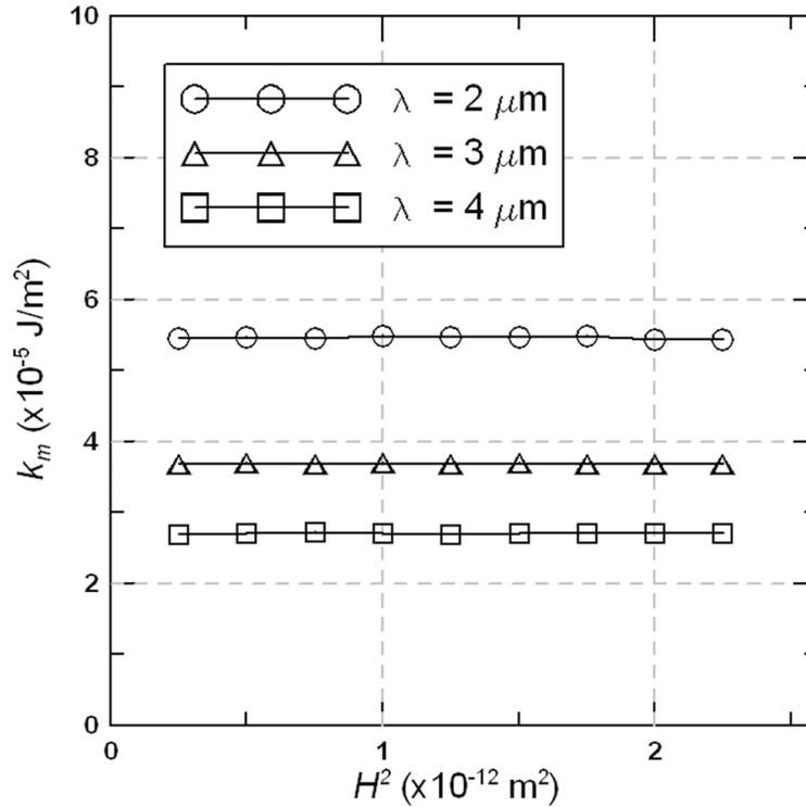
Fig. 4. Variation of  $k_m$  with square of grating height for various values of grating pitch.
