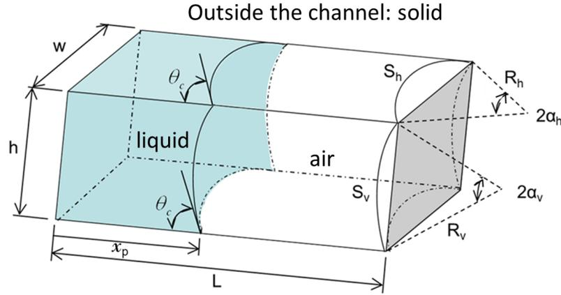
Fig. 1. Schematic illustration of the 3-D model.
