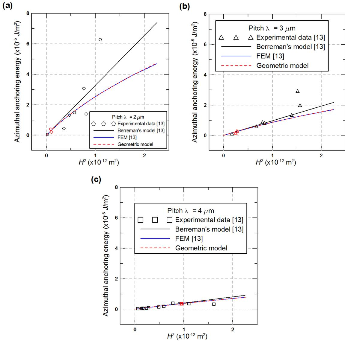
Fig. 5. Experimental and numerical results for variation of surface azimuthal anchoring energy with square of grating height for grating pitches of: (a)  $\lambda = 2 \mu\text{m}$ , (b)  $\lambda = 3 \mu\text{m}$ , and (c)  $\lambda = 4 \mu\text{m}$ .
