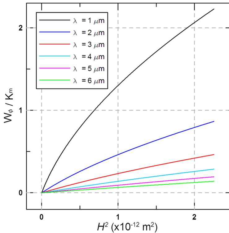
Fig. 3. Variation of  $W_\phi/k_m$  with square of grating height for various values of grating pitch.
