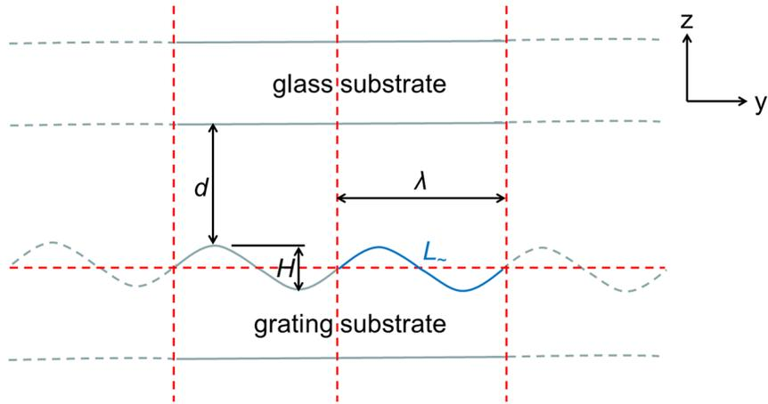
Fig. 2. Schematic illustration of liquid crystal cell structure with sinusoidal relief grating surface.
