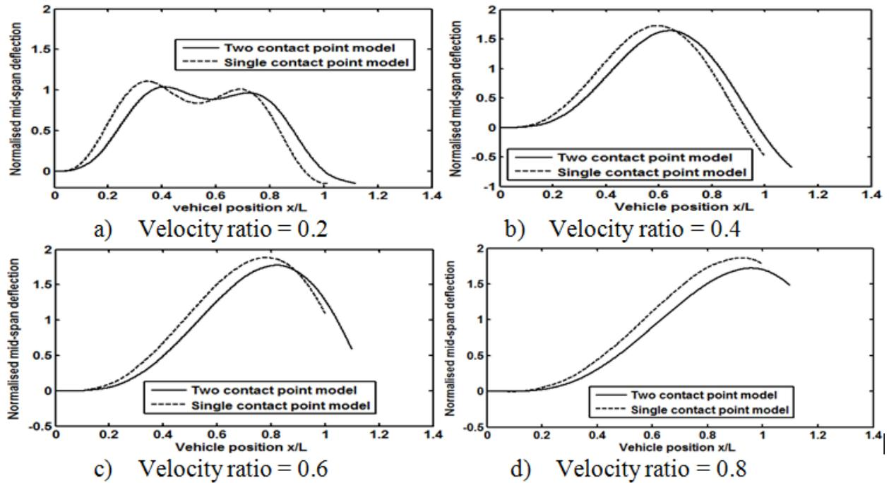
Fig. 7. Bridge mid-span deflection under moving mass condition,  $d = 2$  m ( $d/L = 0.1$ ).
