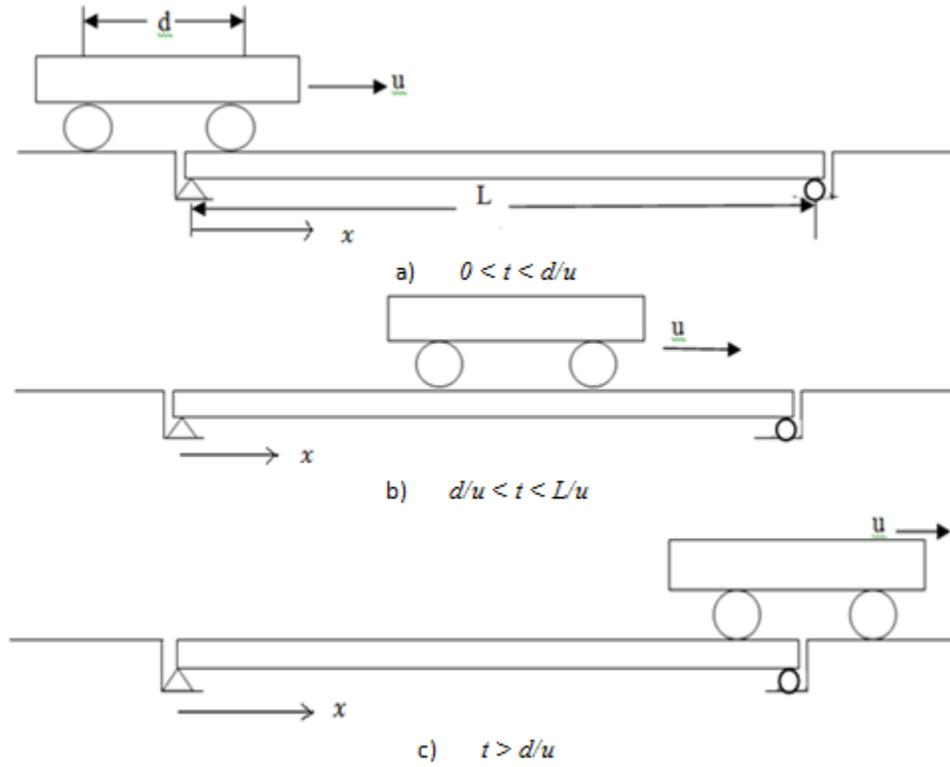
Fig. 2. Three phases of two contact point model.
