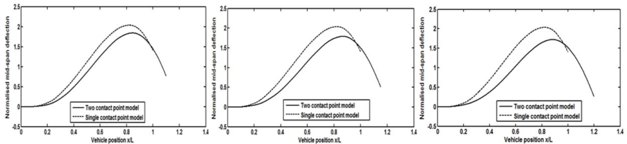
Fig. 5. Bridge mid-span deflection under moving mass conditions (velocity ratio = 0.6).
