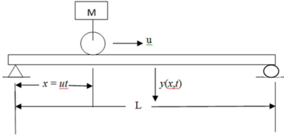
Fig. 1. A travelling mass  $M$  moving on a beam with constant velocity.
