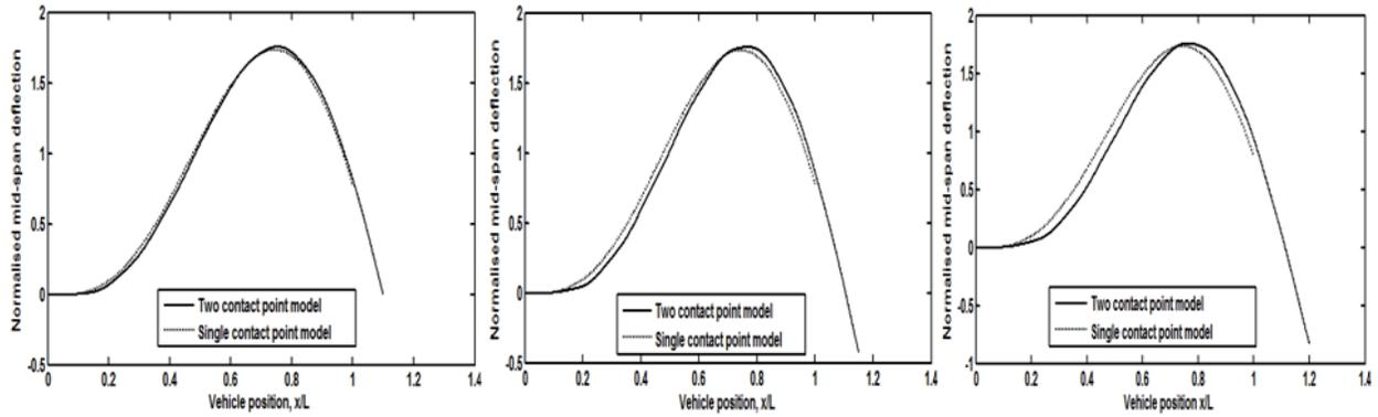
Fig. 4. Bridge mid-span deflection under moving load conditions (velocity ratio = 0.6).
