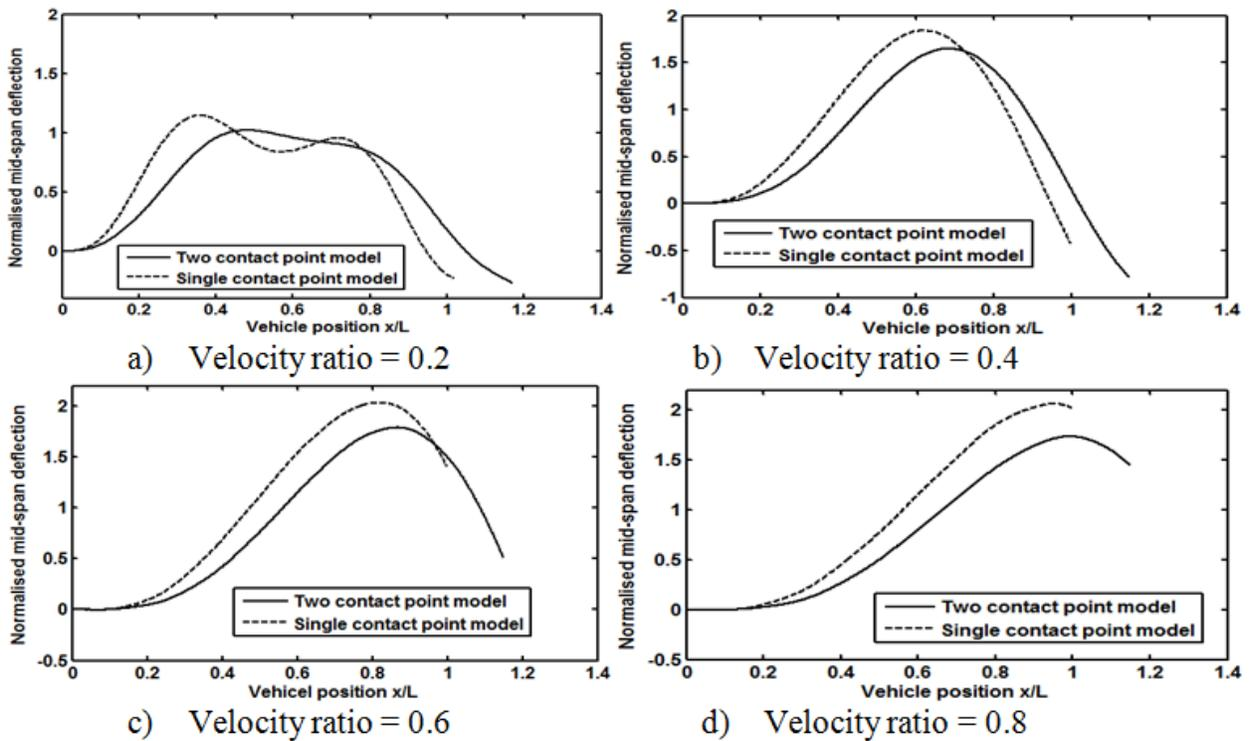
Fig. 11. Bridge mid-span deflection under moving mass condition,  $d = 3$  m ( $d/L = 0.15$ ).
