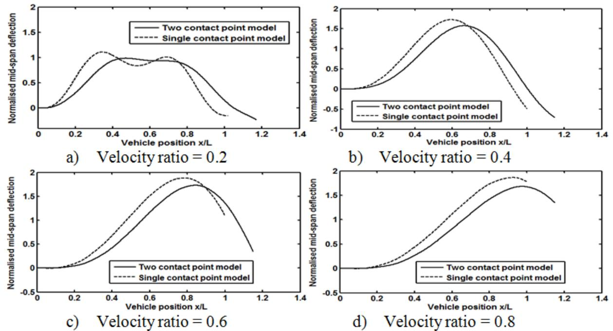
Fig. 8. Bridge mid-span deflection under moving mass condition,  $d = 3$  m ( $d/L = 0.15$ ).
