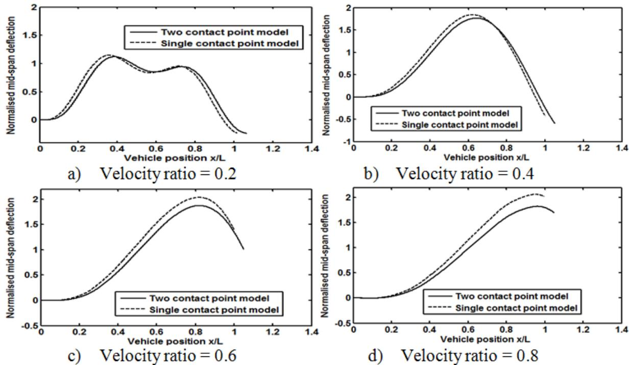
Fig. 9. Bridge mid-span deflection under moving mass condition,  $d = 1$  m ( $d/L = 0.05$ ).
