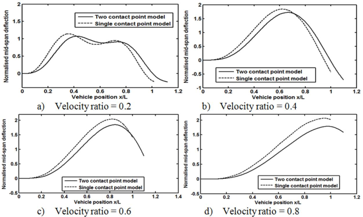
Fig. 10. Bridge mid-span deflection under moving mass condition,  $d = 2$  m ( $d/L = 0.1$ ).
