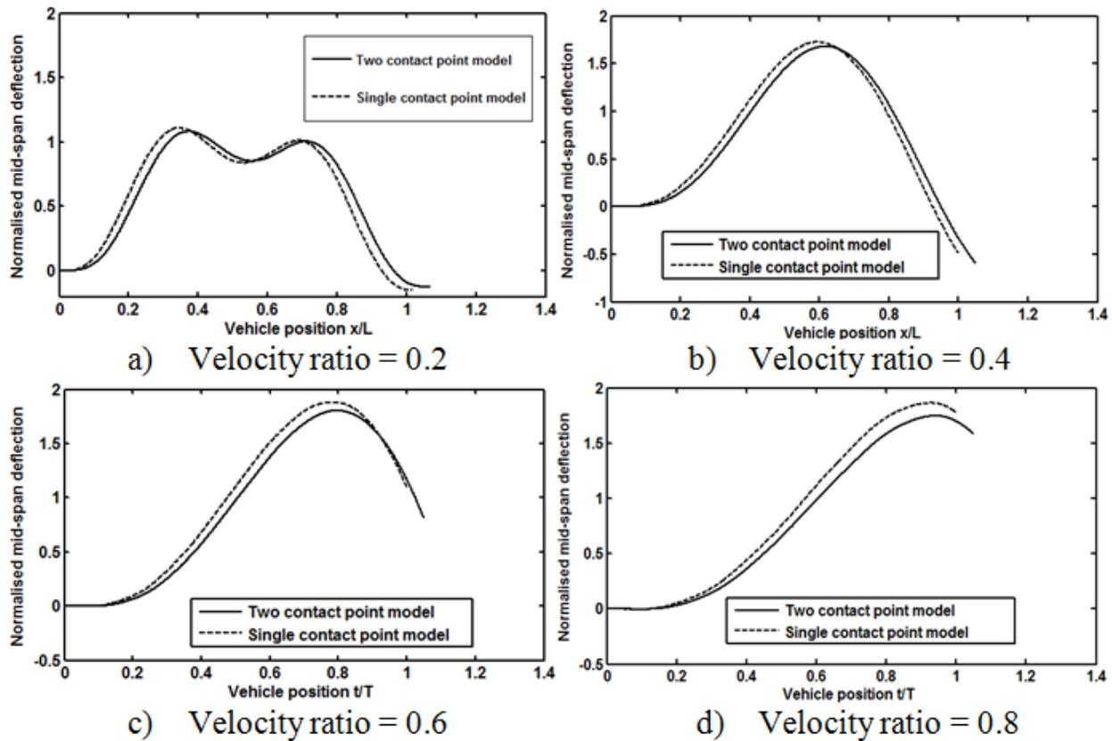
Fig. 6. Bridge mid-span deflection under moving mass condition,  $d = 1$  m ( $d/L = 0.05$ ).
