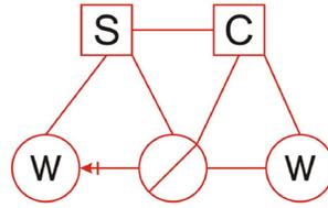
Fig. 1. Functional element representation of a normal bicycle.
