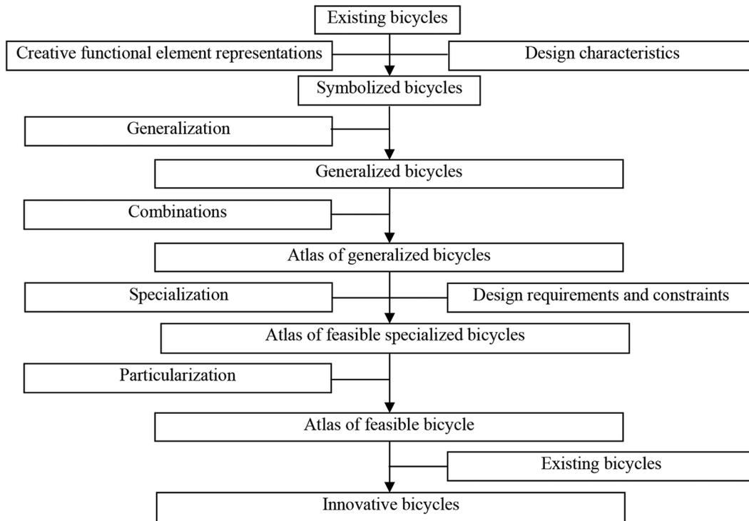
Fig. 2. The design process using functional element representation.
